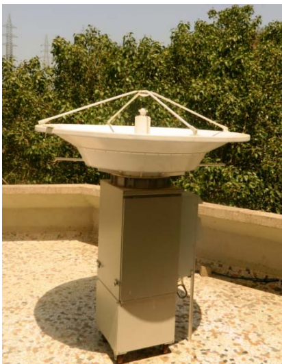
Figure 4. Photograph of ka-band radar for profiling of low level cloud
